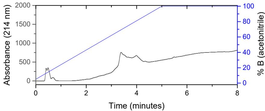
Figure 8—Early eluting compounds (first combined fractions) showing nearly complete removal of the peak eluting at 4.2 minutes in the top run.
