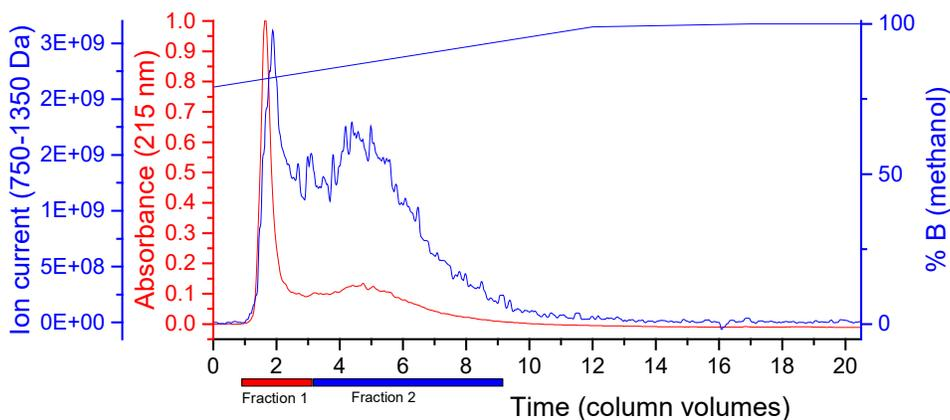
Figure 5—Flash focused gradient on a RediSep Gold C8 column; fractions combined as per the colored bars.
