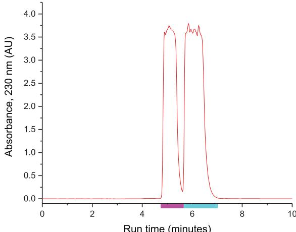
Both isomers were easily resolved with the ACCQ*Prep* HP150 system. Resolution between compounds determines the load capacity for a column. Columns, solvent systems and compounds will determine the actual load for any experiment.
