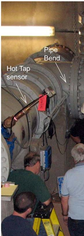
tees, and still yields reliable data. Protruding into the flow stream less than  $\frac{1}{2}$ ", the Hot Tap's sensor tip emits four velocity beams (Figure ), two pointing upstream and two pointing downstream. Each beam is made up of multiple, distinct cells pinged hundreds of times per minute, yielding thousands of velocity data points throughout the water column.
