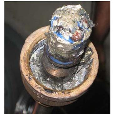
**Sensor tip fouled w/ grease & sludge** after nine months in service
