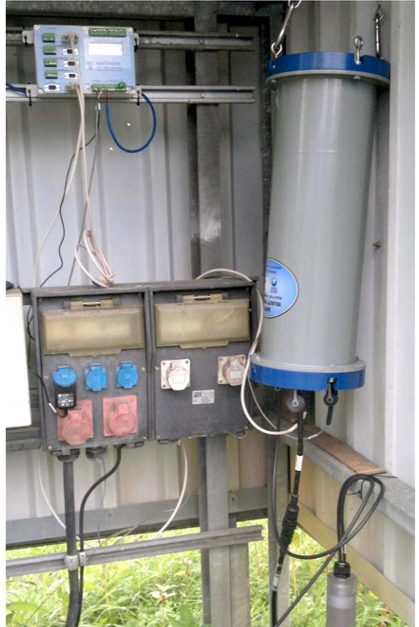
*ADFM Pro20 canister electronics unit (IP68) installed with accQcomm Interface Module*
