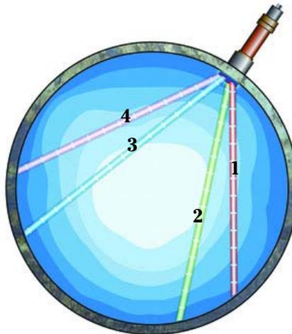
Each data point represents a discrete velocity measurement from an individual "bin" along the Pulse Doppler beam.
