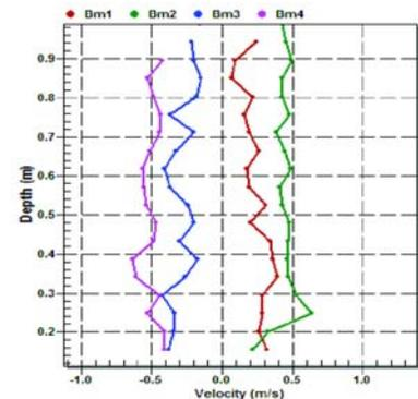
Velocity beams are range-gated, creating individual "bins" to collect data at numerous points throughout the metering section. This ensures that varying velocities within the flow are accurately measured. The chart shows the individual data collected from each beam.
