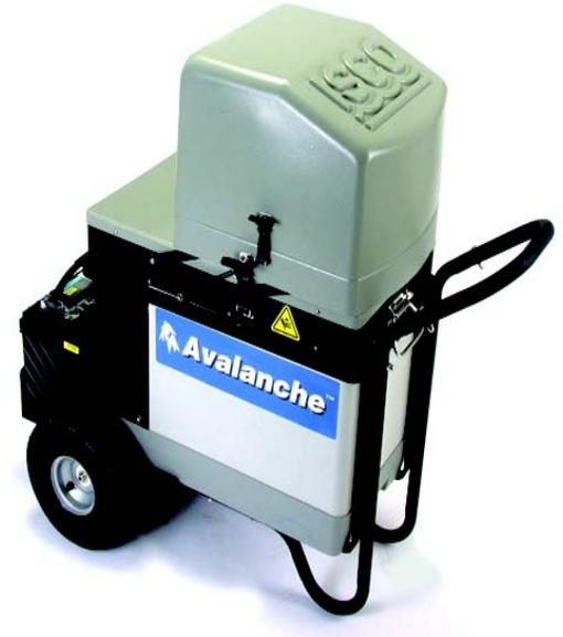
Programs can be initiated via a SMS message as well as enable or disable instructions using text commands. By texting a “6712 STATUS” request to the cellular phone number assigned to the modem, a return message is sent that relays important site information to the end user. This technology is useful in the Storm Water or Discharge Rules Enforcement Monitoring.
