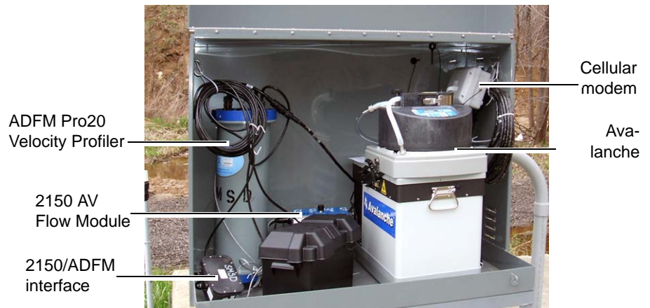
Avalanche sampler in environmental enclosure With cellular modem, ADFM Pro20 Velocity Profiler, and 2150 Area Velocity Module
