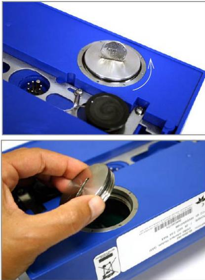
**Figure 3: Removing the SIM cover**
