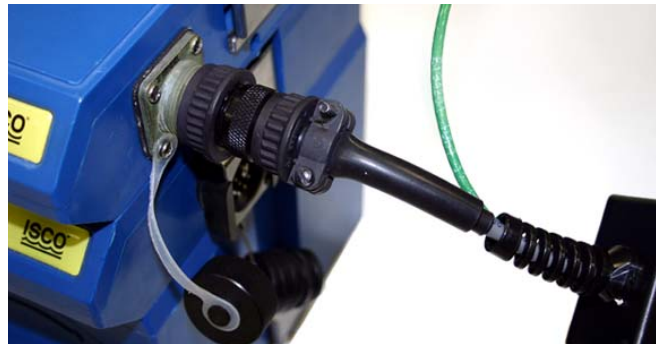
Figure 6: Connect Secondary Protector to 2103
