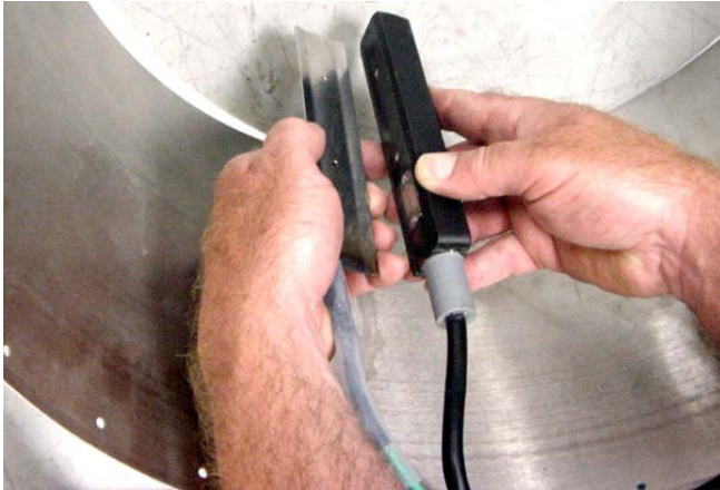
Figure 3: Attach the GEC to the Probe
