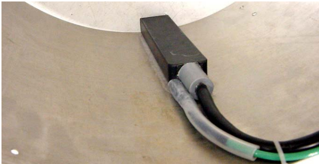
Figure 4: Attach GEC and Probe to Mounting Ring
