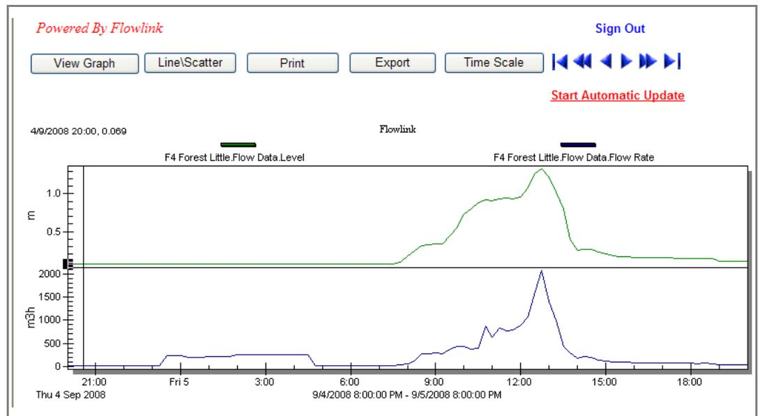
Flowlink WebUI: The web page above displays storm event data from an installation site where the flume's max level was surpassed, but flow was still measured using area-velocity rather than a level-to-flow calculation.
