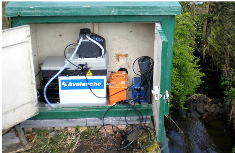
*A typical remote CSO monitoring station with a Teledyne Isco Avalanche refrigerated sampler, multiparameter sonde, and 2105G interface module.*
