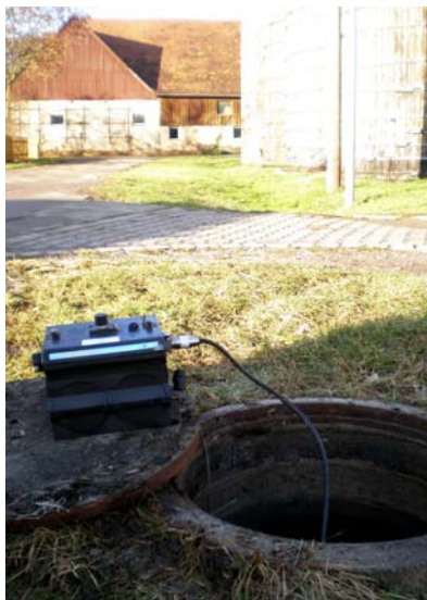
2150EX Flow Logger and Area Velocity sensor installation in pipe. The water seen in the picture is relatively clean, typical of infiltrated water.
