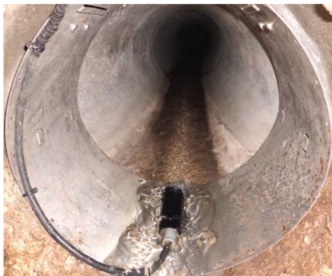
2150EX Flow Logger and Area Velocity sensor installation in pipe. The water seen in the picture is relatively clean, typical of infiltrated water.
