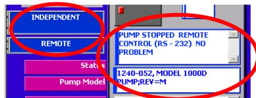
**Figure 4: Status, Pump Model, and Mode Indicators**
