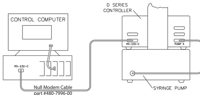
**Figure 1: Serial network connection example**
