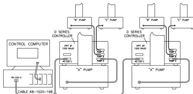
**Figure 2: Serial network connection example**
