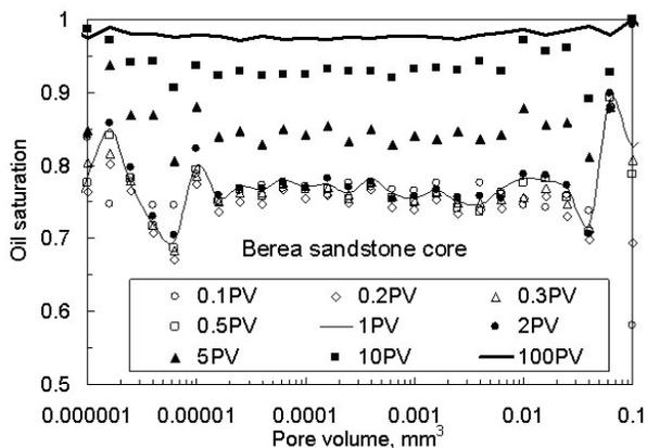
**Figure 4: Oil saturation versus pore size and oil throughput: Berea core**
