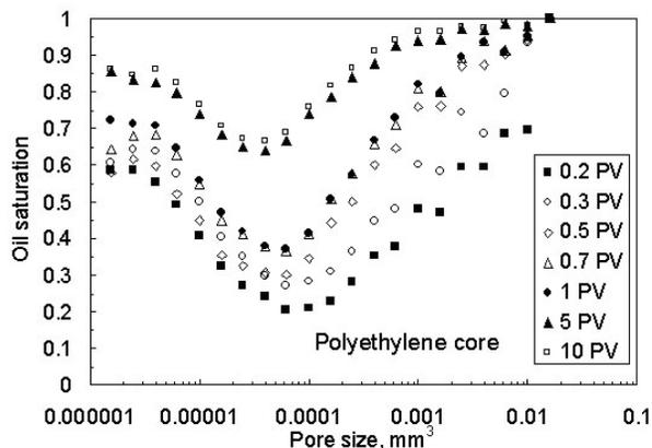
**Figure 3: Oil saturation versus pore size and oil throughput: polyethylene core**
