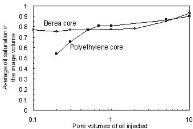
**Figure 2: Average oil saturations in the image volumes versus oil throughput**
