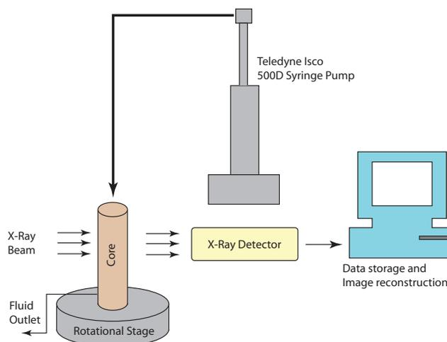
**Figure 1: Diagram of experimental setup**
