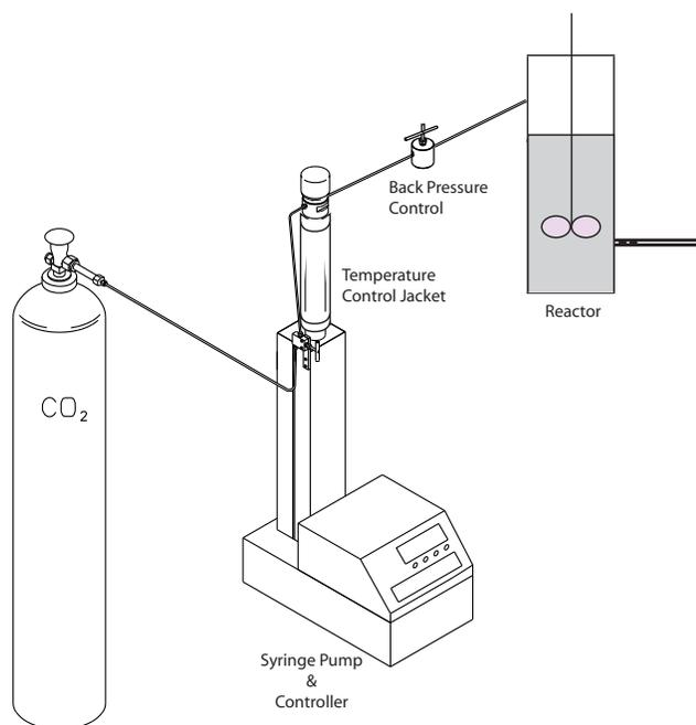
**Figure 3: Configuration for stable mass delivery rate of CO<sub>2</sub> to reactor**
