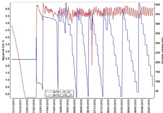
**Figure 4: Recorded evolution of the Teledyne Isco syringe volume (blue line) and apparent volume fraction of hydrogen (H<sub>2</sub>scan specific sensor measurement, red line); the value of 6% for apparent volume fraction of hydrogen corresponds to hydrogen partial pressure of about 60 mbars.**
