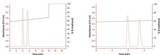
**Figure 3: Original chromatogram; chromatogram modified to reduce run time**
