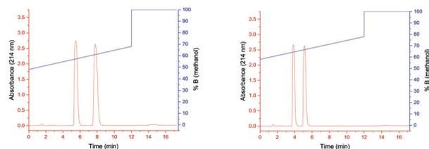
Lower start of gradient by 5% B Raise end of gradient by 5% B
