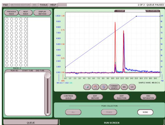
**Figure 1: Display of Post Separation Pause after an injected purification is complete**
