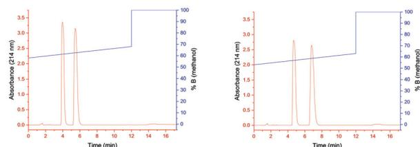
Original chromatogram (58-68% methanol) Lower start and end of gradient by 5% B
