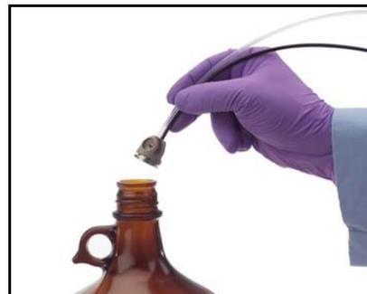
**Figure 2: Remove inlet lines from solvent**
