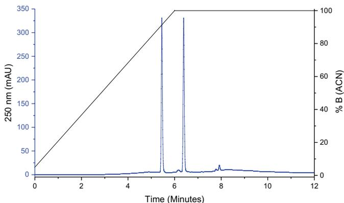
**Figure 1:** Scouting run with 4.6 x 150 mm column and universal test mix in water/acetonitrile. Gradient 5% Solvent B to 100% Solvent B over 6 minutes followed by 6-minute isocratic hold. Due to differences in LC systems, retention times may vary from those shown here.
