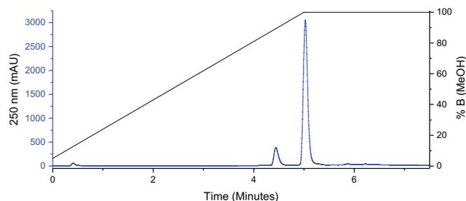
**Figure 2:** Scouting run on 2 x 50 mm column; test mix in water/methanol. Gradient is 5% Solvent B to 100% Solvent B over 5 minutes with a 3-minute isocratic hold at end of gradient. Due to differences in LC systems, retention times may vary from those shown here.
