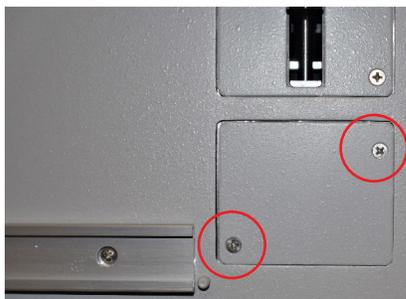
**Figure 1: Panel and location of screws to remove**
