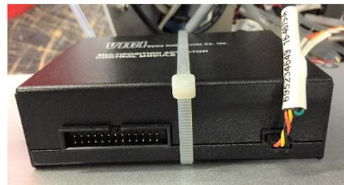
**Figure 9: Large connector on the valve control**
