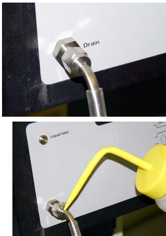
Figure 3-2 Attach drain adaptor; prime with mobile phase if desired
