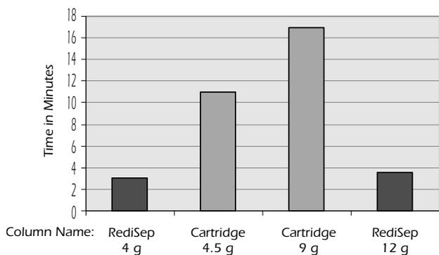
**Figure 4: Time required to elute equivalent sample**
