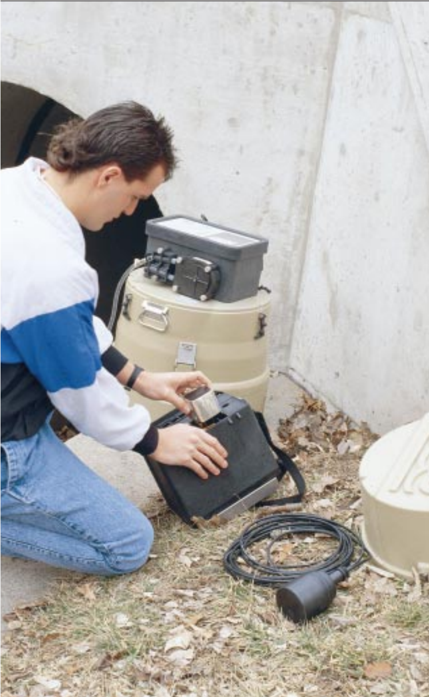
The Isco Flow Logger signals a sampler to collect flow proportioned samples.
