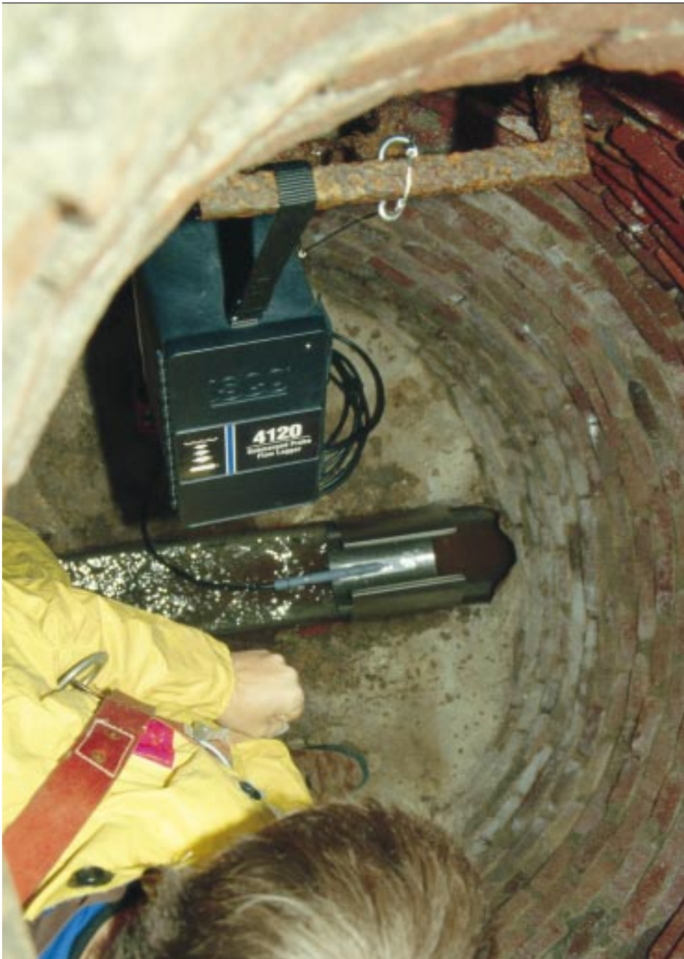
Isco mounting rings make it easy to install the Submerged Probe in round pipes.
