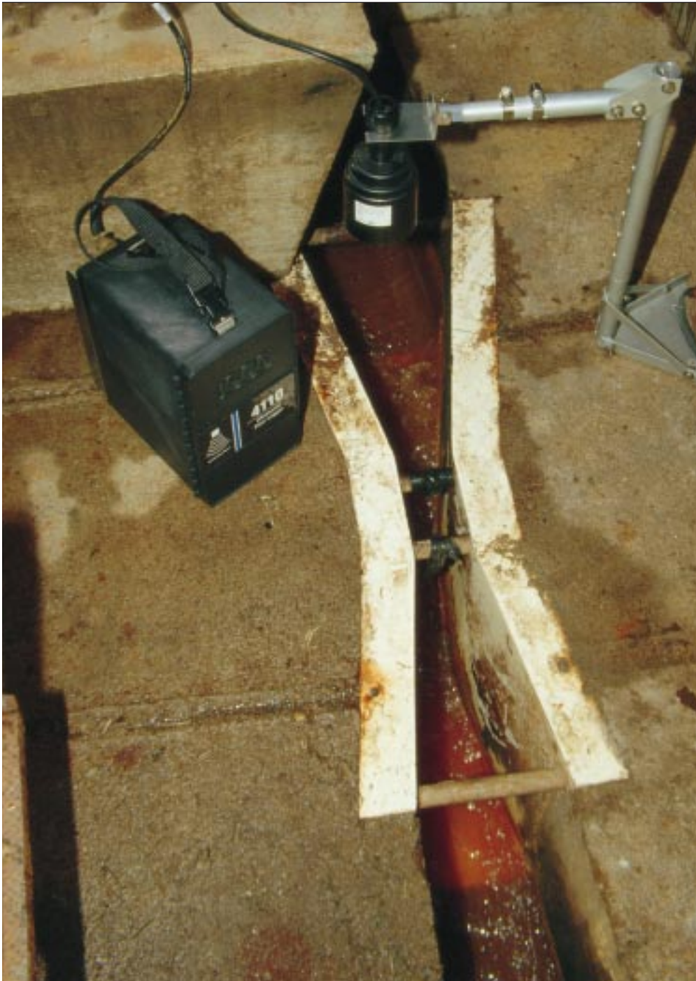
The non-contacting 4110 Ultrasonic Flow Logger accurately measures flow through a Parshall Flume.
