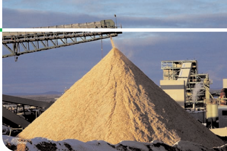
Conveyor belt depositing wood chips.
