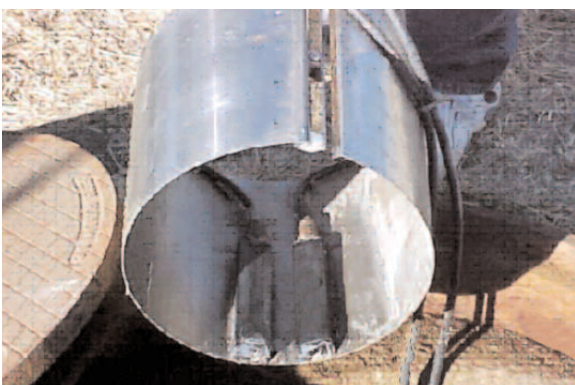
Figure 4. Dual area velocity sensors in mounting ring.
