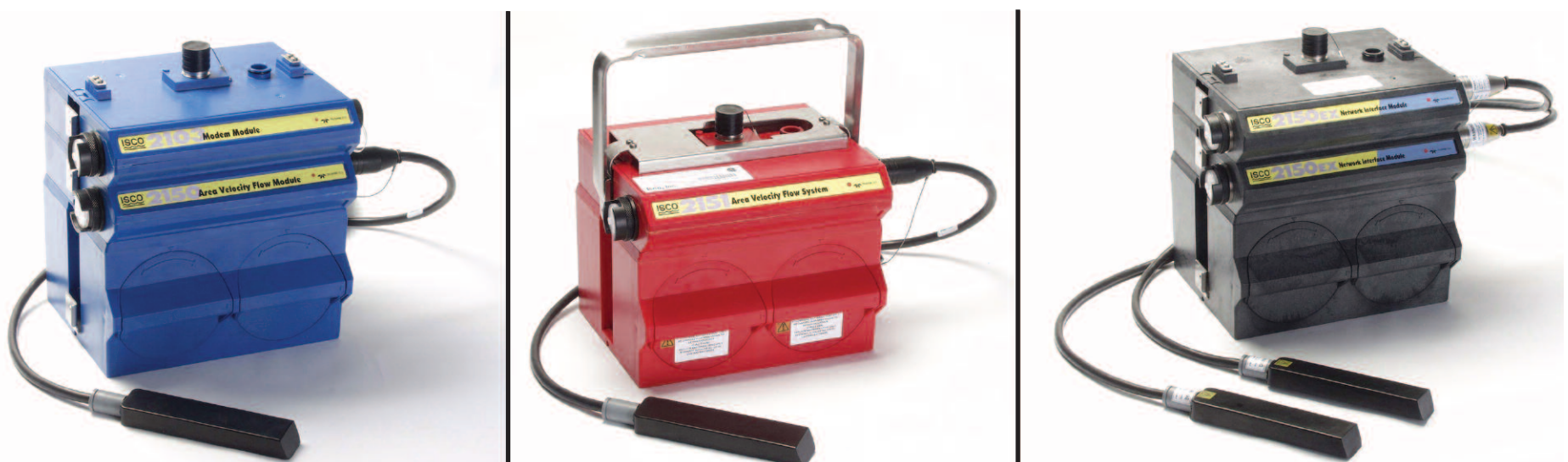
Figure 2. Modular, stackable design of the Isco 2100 Series allows compact configuration for redundant and multi-stream measurements. Left: the standard 2100 Series shown with Area Velocity and Modem Modules stacked on battery module. Centre: the 2151 models are rated for CSA Class 1 Div 1. Right: The 2150EX described in this article is approved under ATEX standard for Zone 0 locations.
