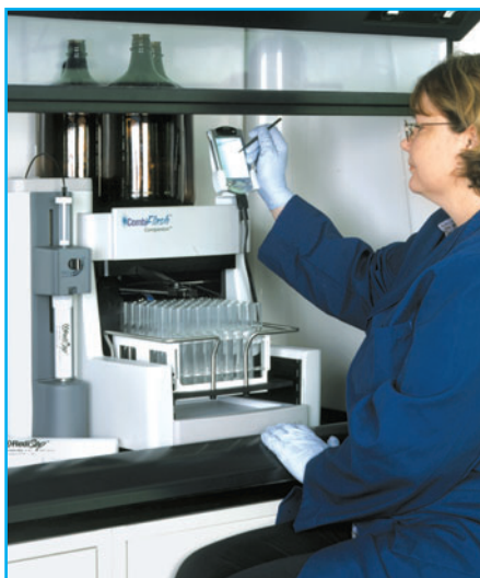
Fig. 3: The Isco CombiFlash Companion fits conveniently in a hood, and includes a lockable mount that holds a standard touchscreen PDA for on-board control via the PDA's browser software.
