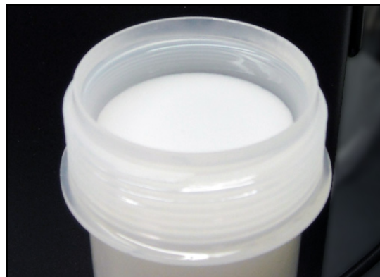
Figure 3: Reservoir Column showing equilibration solvent which requires removal before loading sample
