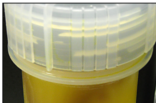
Figure 5: Leakage and Sample Loss Evident around the threads of the reservoir-style column
